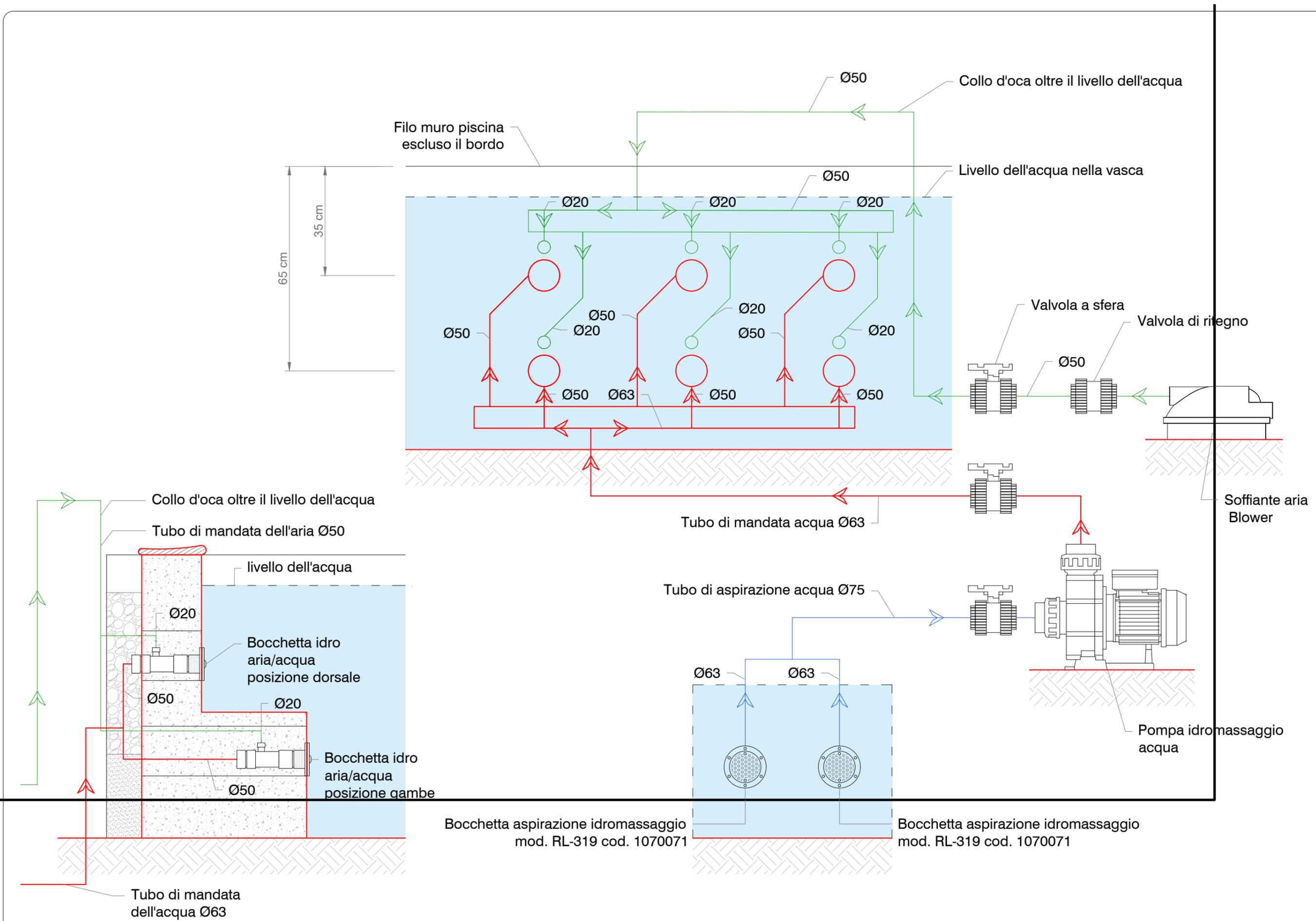
SCHEMA IMPIANTO TIPO KIT IDROMASSAGGIO 6 BOCCHETTE TVENTURI
